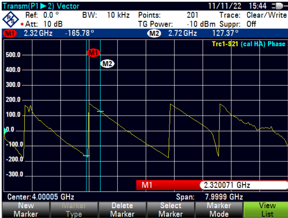
Figure 4. The phase variation of the S 21 characteristics of the ZX60-272LN-S+ with markers showing the specified operating frequency range
