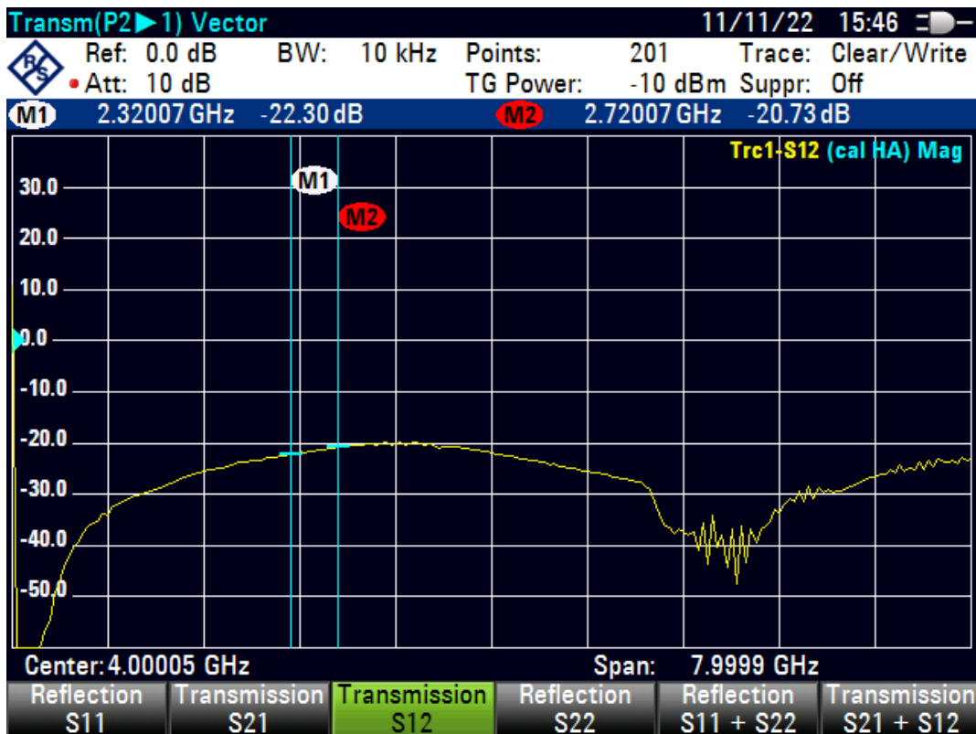
Figure 6. The reverse gain (S 12 ) of the ZX60-272LN-S+
