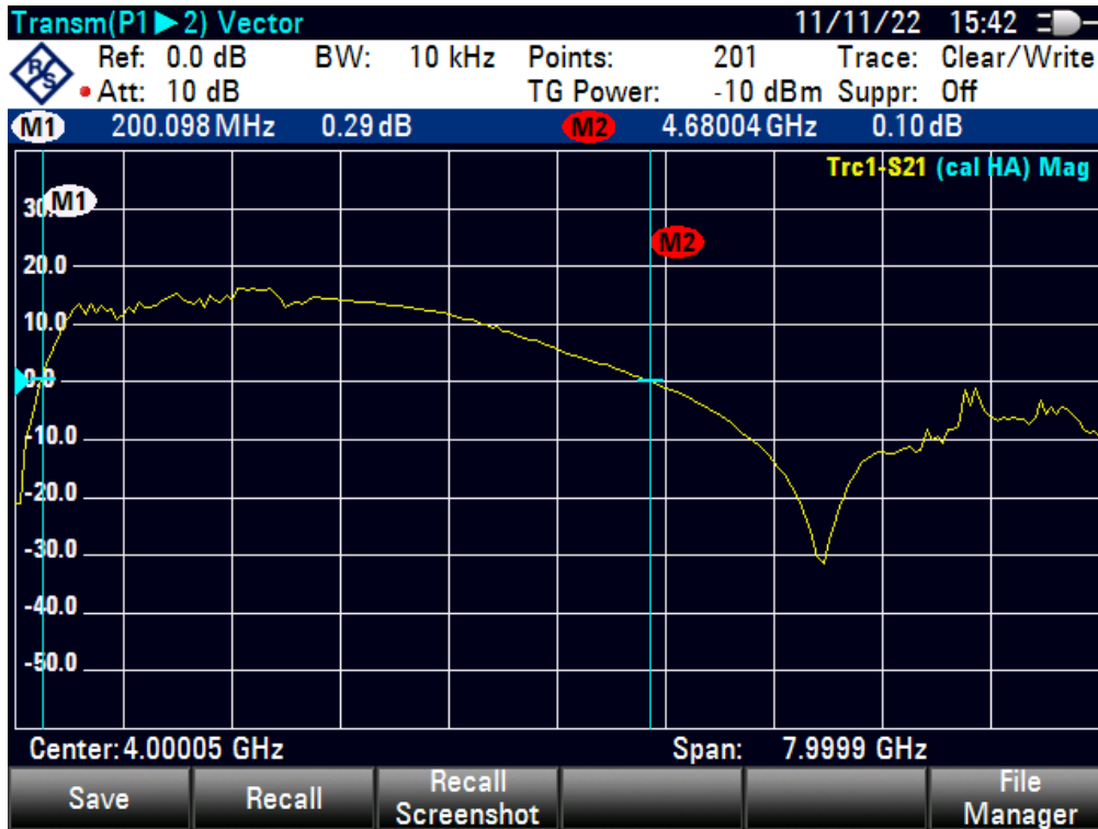
Figure 2. Gain-frequency characteristics of the ZX60-272LN-S+ with markers showing the frequency range where ZX60-272LN-S+ provides gain
