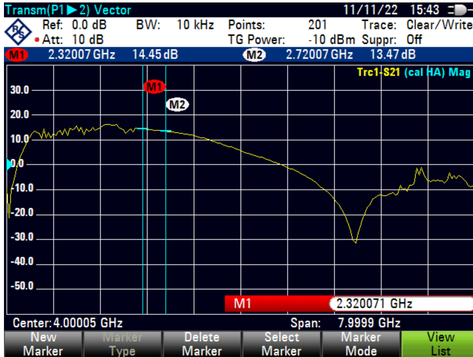
Figure 3. Gain-frequency characteristics of the ZX60-272LN-S+ with markers showing the specified operating frequency range
